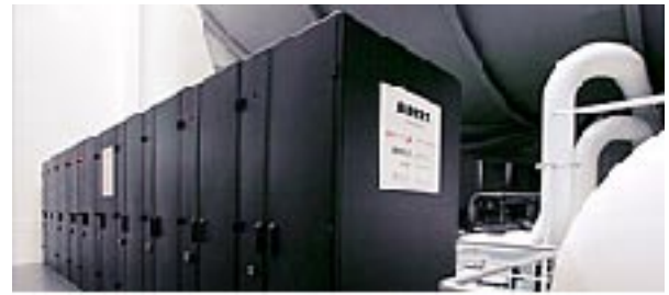
Illustration 2: Albert, the 530-CPU AMD Opteron based HPC used for CFD by Sauber-Petronas (Switzerland, 2004)
